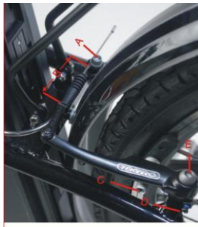
A-Cable clamp bolt B-No contact C-Pad fixing bolt D-Centering screw E-Arm fixing bolt
